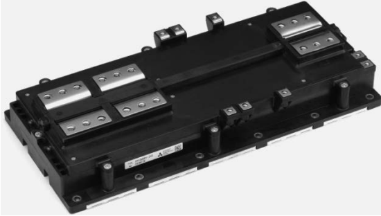
dual switch (Half-Bridge)
