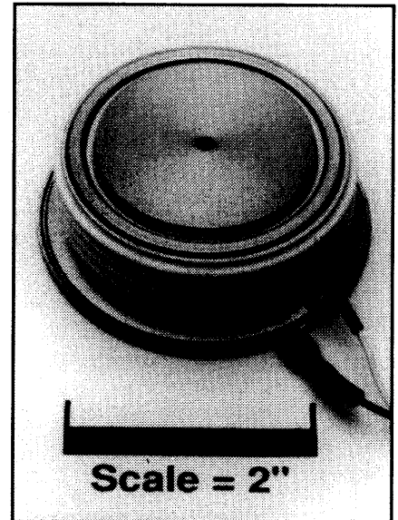
C451 Phase Control SCR 1500 Amperes Average, 2400 Volts
